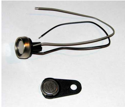
Figure 14. Membership button (bottom) and reader port (top)
